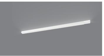
Up-shine cabinet light designed in aluminum shell which provides excellent thermal management. Adopts high efficiency LED. The curved PMMA lens has been used to reach 50°\*100° beam angle. It can be seamlessly connected or seperately installed according to different needs of customers.
