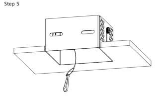
Decorate the ceiling by lime putty after fixing the frame.
