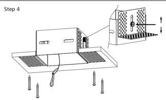
Screwed the frame on the ceiling, the height could be adjust through side screws.
