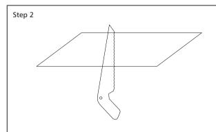
Open a hole on the ceiling according to cutout size of the lamp.
