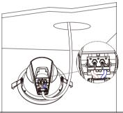
3. Put the main AC wire through line pressing clip, feed the L.N to the fast connection terminal block respectively then compress the line pressing clip.
