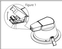
2. Open the line pressing cover, see Figure 1. (Model dependent): Choose the CCT by slide switch, see Figure 2.
