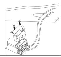
2. Use screw-driver to open the driver terminal cover, feed the main AC wire L. N. in terminal block respectively, then fix the cover back.
