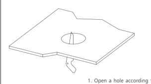
1. Open a hole according to the cutout size of led downlight.
