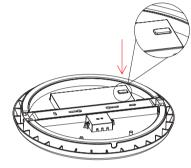
4. Insert rubber stopper back into slide switch properly.
