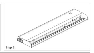
Detach cover of wiring compartment by squeezing its front edge and rotating it backward in its self-hinge.
