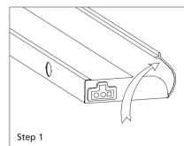
Remove the lens cover from the fixture by lifting its back edge up gently and rotating it toward the front of fixture.
