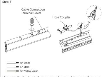
Unscrew the the terminal cover screws by screwdriver, open the cover and punch out the knockout holes, then fasten the hose coupler. Connect the external hose to the hose coupler, thread the power wires through the hose and connect it to the lead wires of lamp by a spiral terminal.
