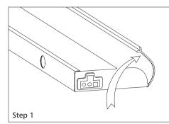
Remove the lens cover from the fixture by lifting its back edge up gently and rotating it toward the front of fixture. See Figure 1. Determine desired location of fixture and mark location of mounting holes (mark at the small end of each keyhole slot).
