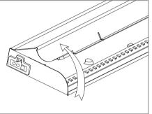
Use a drill gun (or start holes with a awl) and screw in mounting screw in mounting screws at installation locations, ensure the cabinet light securely fixed.
