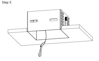
Decorate the ceiling by lime putty after fixing the frame.
