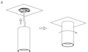
After proper alignment and adjustment between lamp and mounting plate, then rotate the lamp clockwise until it is stuck firmly by mounting plate.
